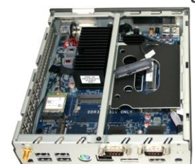
DL20N / DL30N: Passive CPU-Kühlung
